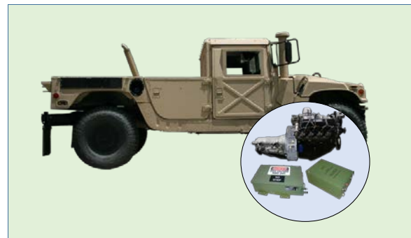
Figure 3: M1152 HMMWV Equipped with DRS 30kW OBVP System
