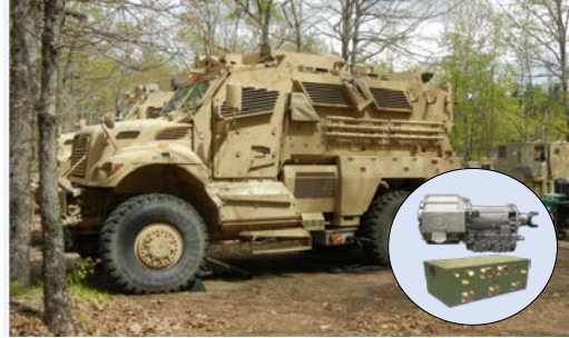
Figure 2: MaxxPro MRAP Equipped with DRS/ATI 3200MSG 125kW OBVP System
